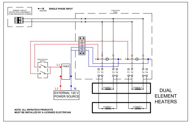
NOTE 3: There will be two Flush Mount Whips in this configuration (one for each heater). In order to have enough wires, only remove the Black #12 wires from both whips and then add the 2 Black #14 wires from each whip packaging to each flex conduit. Then add one Red #14 wire from the contactor panel to each individual whip. Each Flush Mount Whip will contain:
