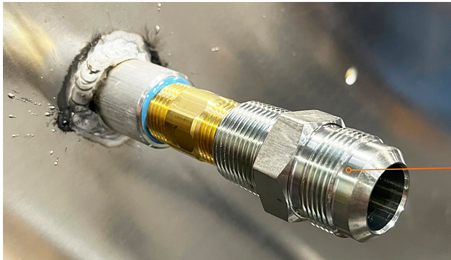
Photo 17: Attaching the Male Flare Hose Adapter
