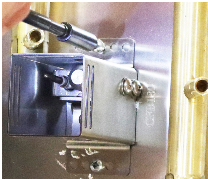
Photo 5: Securing the Pilot to the Plate/Pan
