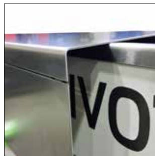
It is easy to produce a closed profile with only one seam.
