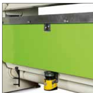
Laser scanner on the folding side, recommended when working from gauging side.
