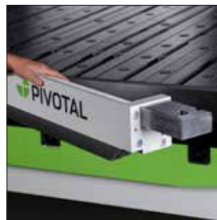
Open the beam when the folding sequence is finished.
