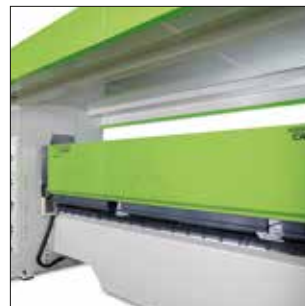
Folding beam in upper position before clamping.
