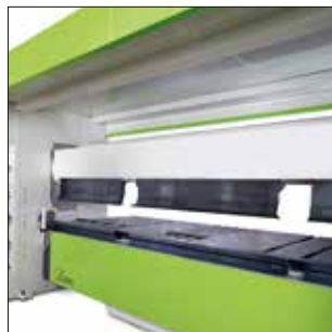
Folding beam in lower position before clamping.
