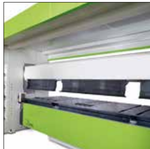
Folding beam in lower position before clamping.
