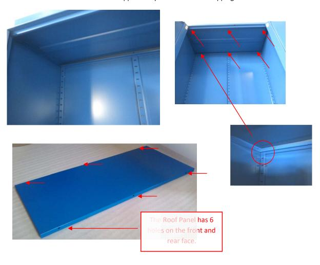
5. Insert the Floor Panel into the lower cavity, ensuring the left and right edge of the Floor Panel is inserted into the side rails. Further secure the cabinet floor with two self tapping screws.
