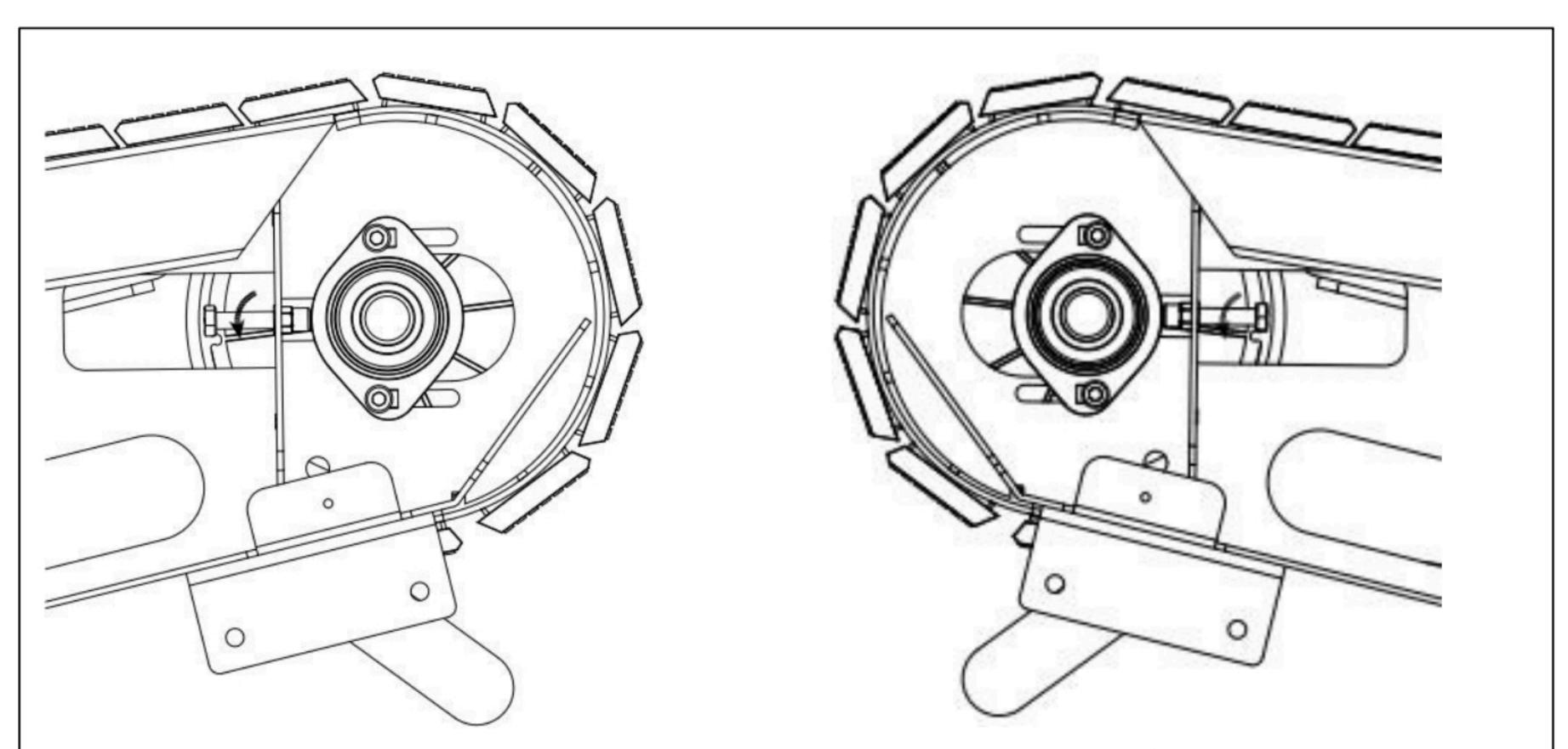
First loosen the two M8 bolts with an 8mm Allen wrench, then tighten / loose them clockwise / counterclockwise with a 14mm open-end wrench, and then tighten the two M8 bolts.
