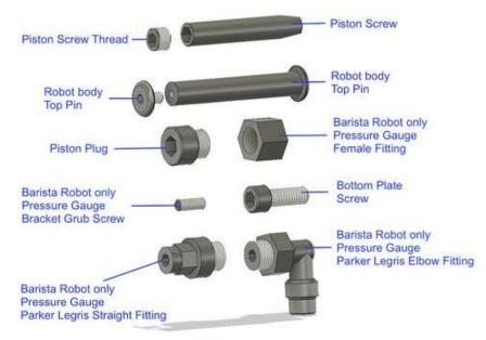
2mm Allen key: Bracket grub screw 3mm Allen key: Top pin 5mm Allen key: Bottom plate screw 6mm Allen key: Piston screw thread, Piston plug 9mm socket: Parker Legris straight fitting 13mm spanner: Female fitting, Parker Legris elbow fitting
