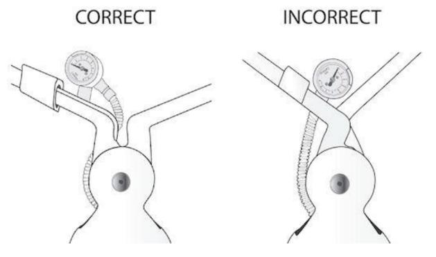
The pressure gauge system is very reliable as long as the tube does not move out of position. If it does move you can easily flick it back to the correct orientation. If the metal sleeve and the flexible tube is being pinched, damaged or broken, please purchase the <u>spare parts</u>. These items are not under <u>warranty</u>.
