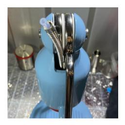
10. Use a H2 Allen key to attach the pressure gauge bracket to the left arm of the Robot.
