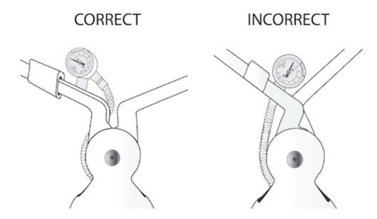
The correct position of the pressure gauge tube is essential for the proper functioning of the pressure gauge system. Ensure that the tube is correctly oriented and securely in place. If it does move, you can easily flick it back into the correct orientation.
