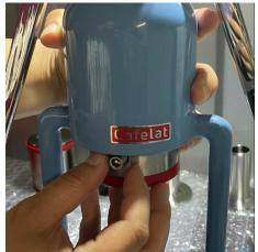
3. To connect the flexible tube to the straight fitting, follow these two stages carefully. In the first stage, the tube should slide in easily for about 5mm. In the second stage, you need to apply much more force to get it to seal, pushing it in another 3mm or so.
