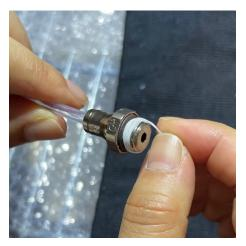
5. To remove the piston screw from the inside of the piston, use an H6 Allen key and unscrew it in a counterclockwise direction.
