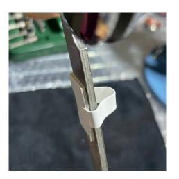
• Put the arm and Teflon rings back in place. If necessary, lay down the Robot to make it easier to work with.
