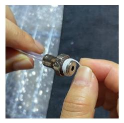
5. Use a H3 allen key to screw the straight fitting.
