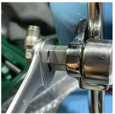
11. Use a 13mm spanner to install the straight fitting back on the gauge.
