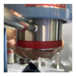
2. Remove the piston screw from the back of the Robot by pinning it out.
