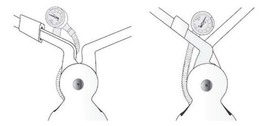
The correct position of the pressure gauge tube. The pressure gauge system is very reliable as long as the tube does not move out of position. If it does move you can easily flick it back to the correct orientation.
