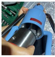
10. Insert the screw into the back of the robot. Use an H5 Allen key to tighten the piston screw thread.
