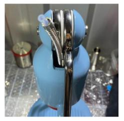
5. Remove the piston screw thread using a H5 Allen key. Then carefully remove the piston screw from the back of the robot by carefully pinning it out.
