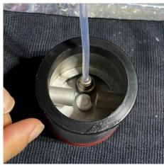
9. Line up the holes in the arm lever and piston. Carefully insert the piston back into place.
