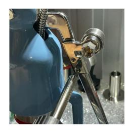
3. Remove the flexible tube from the elbow fitting by pulling the collar of the elbow fitting while simultaneously pulling the tube away from the fitting.
