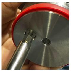
8. Wipe the piston thread hole area clean. Then use an H6 Allen key to install the piston blanking plug and Teflon washer into the piston.
