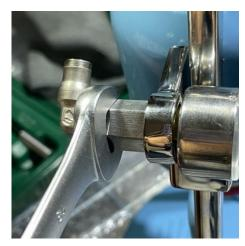
2. Take out the metal sleeve. Remove the pressure gauge bracket by using a H2 Allen key.
