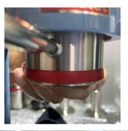
4. Remove the piston screw from the back of the Robot by pinning it out.
