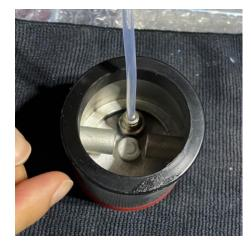
11. Put the piston back. Line up the arm lever and piston holes.
