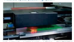
0 四路光源可调,光源强度可调,光照均匀,采集图像更趋完美; 可很好的识别(包括凹凸不平的Mark点),适应镀锡,镀铜, 镀金,喷锡,FPC等各类型不同颜色的PCB。 Adjustable four light sources, light intensi ty is adjustable, lightis uniform, and image acquisition is more perfect; Good identification (including uneven mark points), apply for tinning, copper plating, Gold plating, tin spraying, FPC and other types of PCB with different colors.
