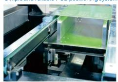
0 可编程弹性侧夹和磁性支撑装置。 Programmable elastic side clamp and magnetic supporting device.
