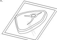
2. Place the open end of the bag across the Vacuum Compartment Seal Gasket, making certain that the open end is within the Vacuum Channel.
