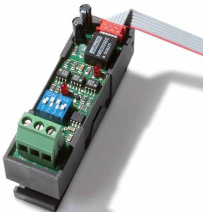
ICI-485 module required to connect VISY-Input / VISY-Output
