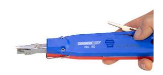
With the Sensor No. 40, wires with a conductor diameter of 0.35 - 0.9 mm and a wire diameter of 0.7 - 2.6 mm can be wired into LSA panels or blocks. With a gentle push on the tool, the wires are inserted and cut off in just one single step. Manual stripping or screwing is not required.
