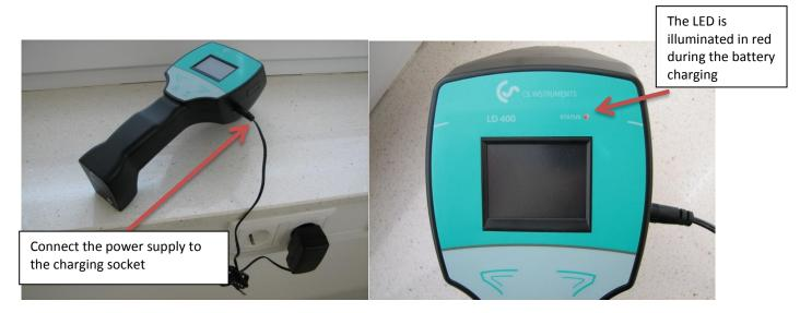
The LD400 checks the charge status of the battery and automatically starts the charging process. The following scenarios are possible:
