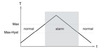
A switchover delay time ( $t_{DS}$ ) can be applied to the switchover to the alarm state. Equally, one switch-back delay time ( $t_{DR}$ ) of several can
