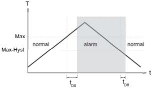
be applied to switching back to the normal state.
