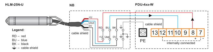
In the case using a connection box with integrated overvoltage protection, the sensor needs to be connected to the bottom series of terminals. This series of contacts is marked by label SENSOR.
