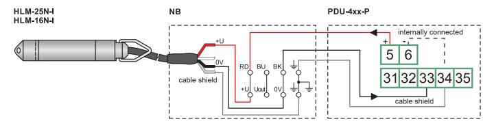
In the case using a connection box with integrated overvoltage protection, the sensor needs to be connected to the bottom series of terminals. This series of contacts is marked by label SENSOR.
