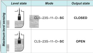
For security reasons, we recommend to use **SO variant** (normally open, sensor closes when immersed) for **minimum level detection**. Any failure of the sensor or wiring is equally apparent as the emergency level state. Analogously – for the **maximum level detection** is recommended to use **SC variant** (normally closed, sensor opens when immersed).
