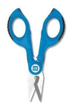
For cutting and stripping of Cu/Al conductors as well as for crimping of terminals from 0.5 to 4 mm². The cutting edges of the scissors are serrated. This achieves a flush cut and the slipping of the cable is prevented.
