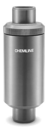
Chemline **SV Series** vacuum breaker valves are designed as one way valves, opening only when process pressure drops in order to allow air/gas into the process. Its operation is simple as the ball is held at the top of the vertically mounted valve by a coated spring.
