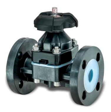
The Chemline HD Series HYBRID diaphragm valve is a composite valve with a steel core fully lined with PFA or PVDF. These valves are used for sanitary and high purity applications as well as aggressive chemicals. Diaphragm valves are designed for throttling. They are perfect for a composite (fibreglass), alloy or lined steel piping. The plastic/metal hybrid construction offers the chemical resistance and toughness of plastic along with the strength of metal.
