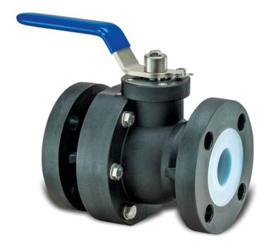
The Chemline HB Series HYBRID ball valve is a composite valve with internal steel reinforcement, fully lined with PFA or PVDF. These full port valves are perfect for composite, alloy or lined steel piping. The plastic/metal hybrid construction offers the chemical resistance and toughness of plastic along with the strength of metal.
