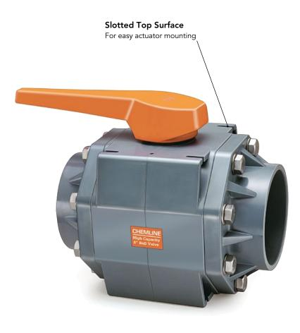
Chemline **HC Series** is a true large port 6" ball valve manufactured in PVC, polypropylene and PVDF. Most other 6" valves often are 4" with ends increased to 6". HC Series offers an unobstructed full port which allows passage of mechanical pipe cleaners or "pigs". Applications include unfiltered sea water and sewage lines. It is also suitable for mild slurries and vacuum lines.
