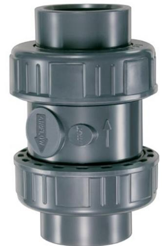
Chemline **ES Series** PVC True Union Spring Check valves have a PTFE covered stainless steel spring for positive closing. Compared to ball check valves, ES Series require very low liquid head pressure to close. That means more flexibility as to where valves may be placed in a piping system.
