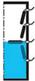
Fixed on the walls of the tanks using a stuffing box.
