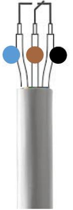
The liquid reaches the float which by tilting gives the signal to the pump to start for emptying
