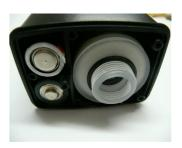
Two AA 1.5 volt Alkaline Batteries Type MN1500, LRG 1.5 or similar must be installed in the TEK-OX to the correct way to enable it to operate.
