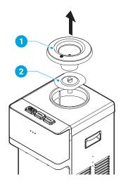
F. Remove the bottle support collar (1) from the top of the dispenser, then the white separator (2) covering the cold water reservoir. Dampen the cloth with some of the solution and wipe the bottle support collar and white separator clean, then wipe or rinse them with fresh hot tap water. Set aside to air dry.
