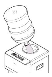
G. Pour the cleaning solution into the empty cold water reservoir. (Solution will drain down into hot water reservoir.) Be sure to fill the cold water reservoir all the way to the top. If necessary, prepare more solution. Allow solution to sit for 20 minutes, then drain the reservoirs as described in step C. Rinse out the solution bottle or bucket, then fill with 2 gallons of fresh hot tap water and refill the reservoirs.
