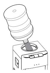
G. Pour the cleaning solution into the empty cold water reservoir. (Solution will drain down into hot water reservoir.) Be sure to fill the cold water reservoir all the way to the top. If necessary, prepare more solution. Allow solution to sit for 20 minutes, then drain the reservoirs as described in step C. Rinse out the solution bottle or bucket, then fill with 2 gallons of fresh hot tap water and refill the reservoirs.
