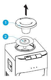
top of the dispenser, then the white separator (2) covering the cold water reservoir. Dampen the cloth with some of the solution and wipe the bottle support collar and white separator clean, then wipe or rinse them with fresh hot tap water. Set aside to air dry.
