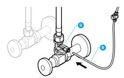
**E.** Gently tug on the tube (B) to ensure a secure connection with the feed water adapter (G).
