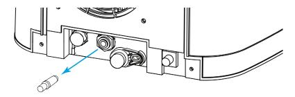
**B.** Insert the elbow-connector end of the Shutoff Valve Tube (A) into the Water Inlet (10). Secure with Locking Clips (E) if desired.
