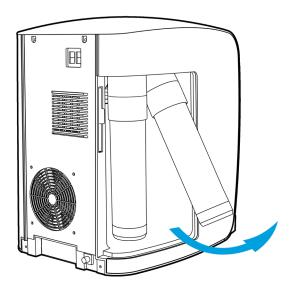
A. Connect the filter to the Filter Housing (D) by inserting the filter and rotating clockwise until the BRIO logos on the filter and the Filter Housing (D) are aligned.
