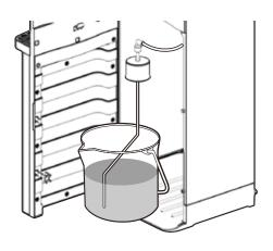
E. Insert the bottle adapter tube into the bottle or bucket with the solution, secure the cap if using a bottle, and slide into dispenser, shutting door securely.
