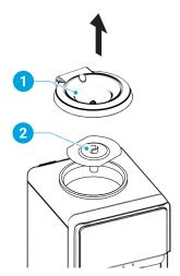
F. Remove the bottle support collar (1) from the top of the dispenser, then the white separator (2) covering the cold water reservoir. Dampen the cloth with some of the solution and wipe the bottle support collar and white separator clean, then wipe or rinse them with fresh hot tap water. Set aside to air dry.
