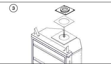
Install the 8" gasket and your chimney supplier's insulated chimney anchor plate.
