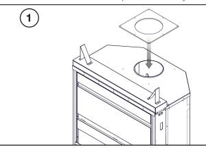
Install the 10" anchor plate gasket concentric to the flue collar.
