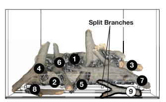
Place log #9 on the media tray in between the third and fourth grate posts. Ensure the split branches face to the left. Apply charcoals to any visible spaces along the front of the media tray (not illustrated).
