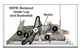
5. Place the bumpout on log #5 into the notch in log #1, resting the opposite end along the front grate.
