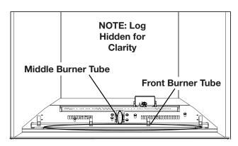
1a. Apply glowing embers to the middle and front burner tubes (not illustrated). \*
