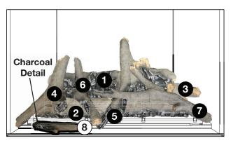
8. Place log #8 on the media tray in between the first and second grate posts. Ensure the charcoal detail faces to the left.
