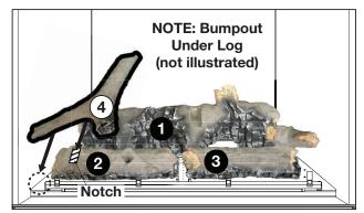
4. Place the bumpout on log #4 into the notch in log #2, resting the opposite end beside the first grate post.
