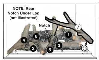
7. Place the left side of log #7 into the notch in log #5. Rest the rear notch in log #7 on the fourth grate post.
