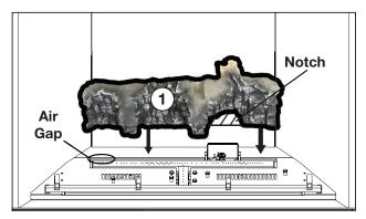
Place log #1 at the back of the burner, ensuring the notch fits around the pilot shield and is pulled forward tight behind the pilot shield. Do not cover the air gap behind the burner.
