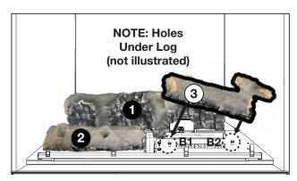
3. Place the holes in log #3 on B1 and B2.
