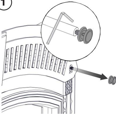
Loosen set screw, unthread and remove the decorative bypass pull knob.
