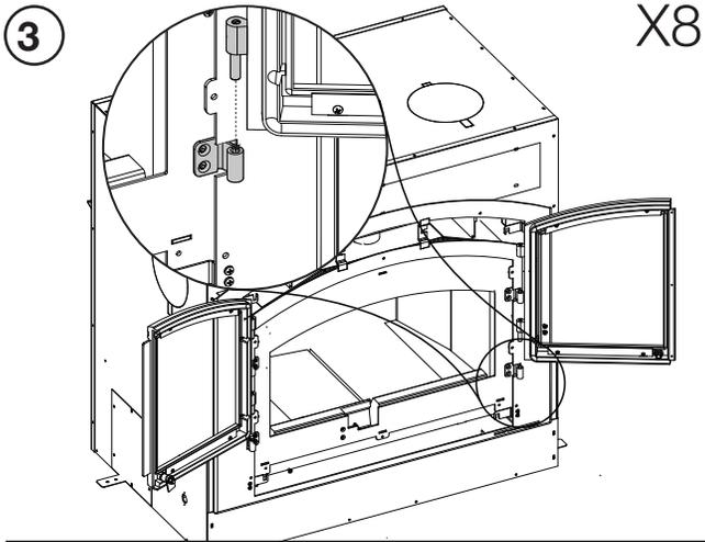
3 Open both doors and remove by loosening set screws on hinges and lifting up until the hinge pins clear the door hinges. Set aside.
