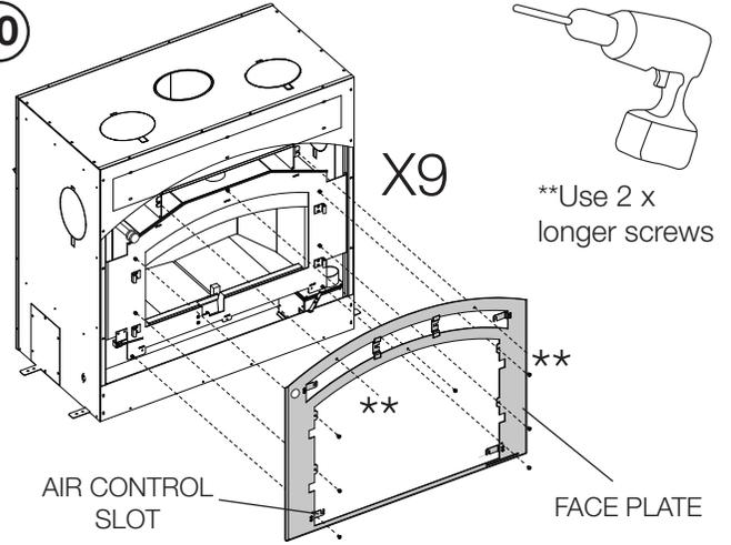
Reinstall the face plate using the 9 screws removed in step 4.
