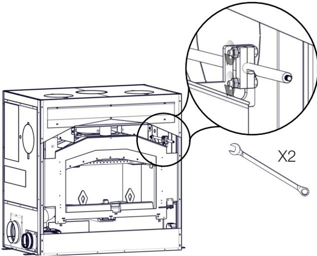
Fully tighten both nuts until the stopper blocks are completely secure around the bypass damper rod. Ensure the stopper blocks do not move.
