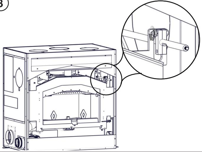
Install one nut and hand tighten to hold stopper blocks in place. Repeat for bottom screw, lockwasher and nut.
