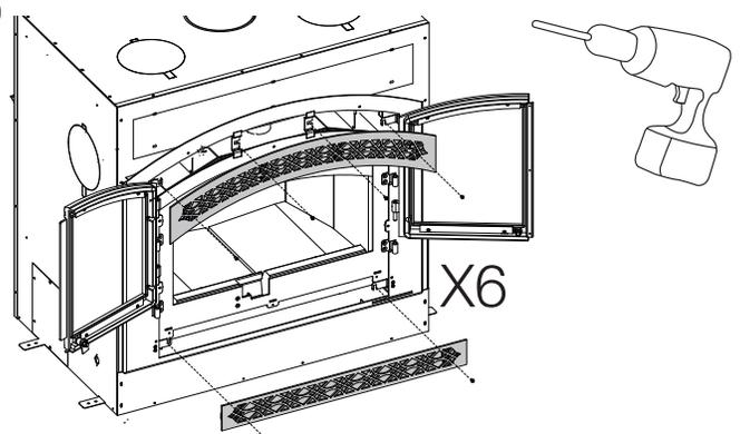
Remove the 4 screws securing the top inset to the appliance. Remove the 2 screws securing the bottom inset to the appliance.
