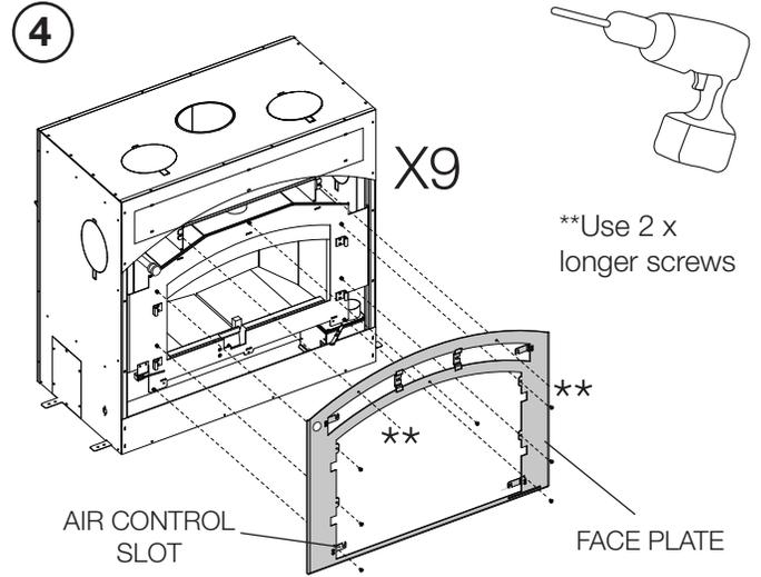
4 Remove the 9 screws securing the face plate to the appliance.
