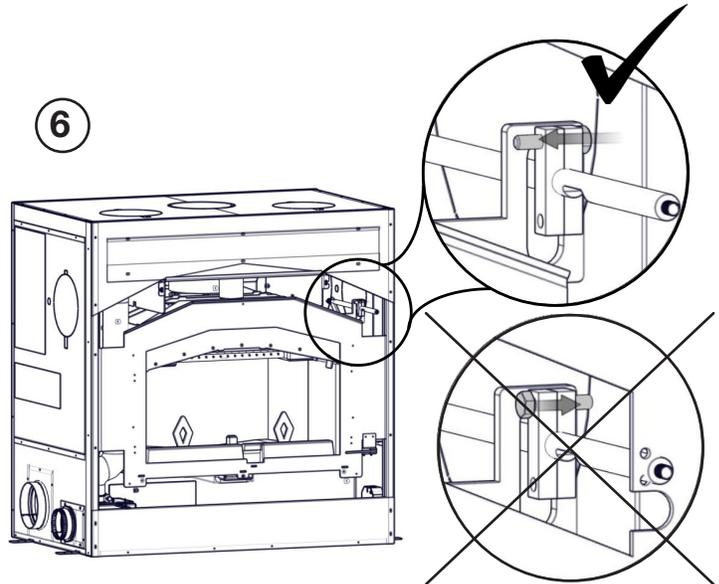
6 Install one screw into the top hole of stopper blocks.
