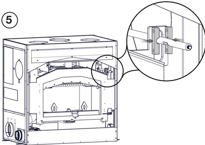
5 Install two stopper blocks around the bypass damper rod.
