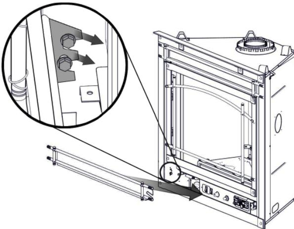
LIFT AND SLIDE THE BOTTOM MESH ASSEMBLY OVER THE REMAINING SHOULDER BOLTS UNTIL IT COMES TO A STOP.
