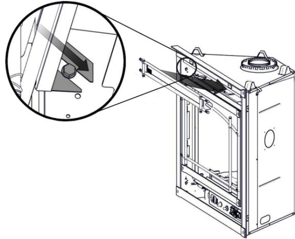
LIFT AND SLIDE THE TOP MESH ASSEMBLY OVER THE TOP SHOULDER BOLTS UNTIL IT COMES TO A STOP.
