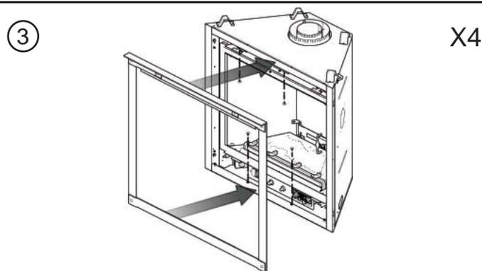
LINE UP THE SLOTS IN THE SECURING BRACKETS OF THE OUTSIDE TRIM ASSEMBLY WITH THE HOLES IN THE TOP AND BOTTOM OF THE APPLIANCE AND SECURE USING THE 4 #8 X 3/8" SCREWS PROVIDED.
