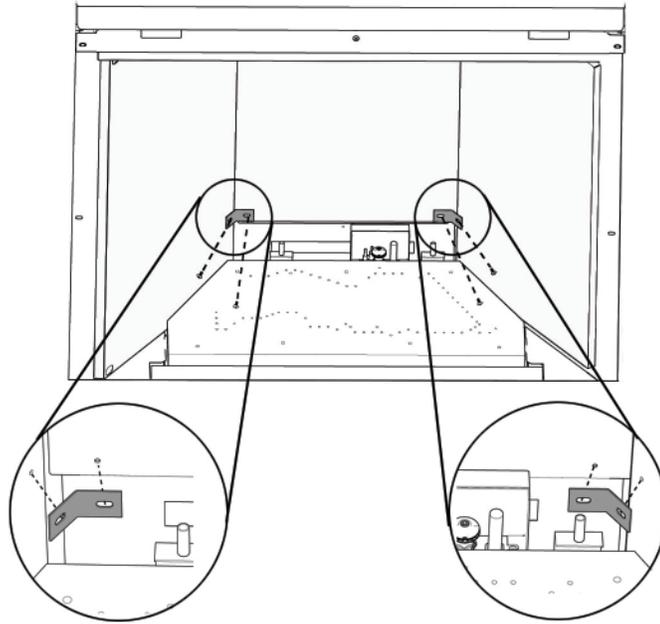
NOTE: PLACE BRACKETS IN BOTTOM CORNERS BETWEEN SIDE AND REAR PANELS
