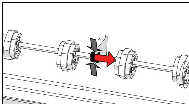
4. Remove the bushings from the bracket by pinching them and pushing them toward the right. Remove the flicker rod.
