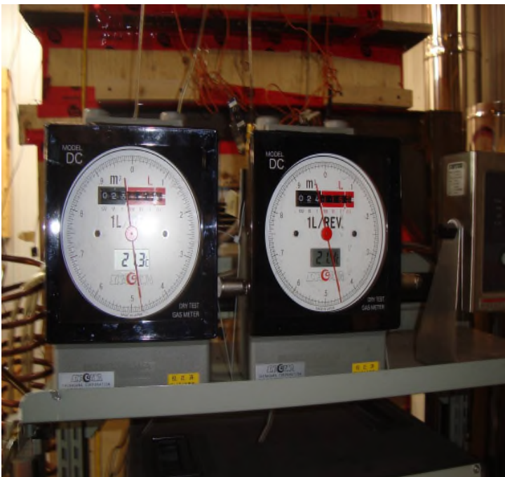
Picture 11: Dry gas meter
