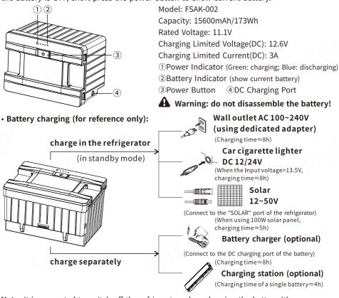
**Note:** It is suggested to switch off the refrigerator when charging the battery (the power supply may mainly power the compressor when the refrigerator is running).
