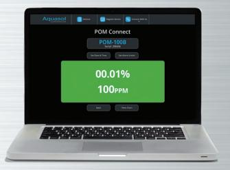
**GREEN** indicates that the current measurement is lower than the "Lower Alarm Limit."
