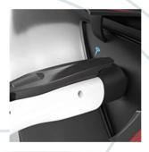
Step 3: Confirm Tesla vehicle's indicator turns green
