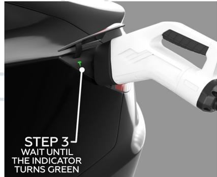
**DISCONNECTING:** Disconnect **ONLY** after charging is complete. Always disconnect the adapter from your vehicle first by pulling the charger handle and adapter together (**DO NOT** press unlock button on charger handle), then disconnect it from the charging station.
