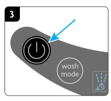
Press and hold the "Power" button for 3 seconds to turn on the Bottle Washer Pro®.
