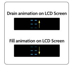
The machine will start by draining the sump to make sure it starts with clean water, then it will begin filling the sump and heating the water.
