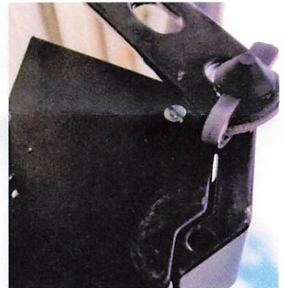
PIN FOR LINKAGE BAR CONNECTION (MAKE SURE PIN IS ATTACHED IN THE TOP HOLE.)
