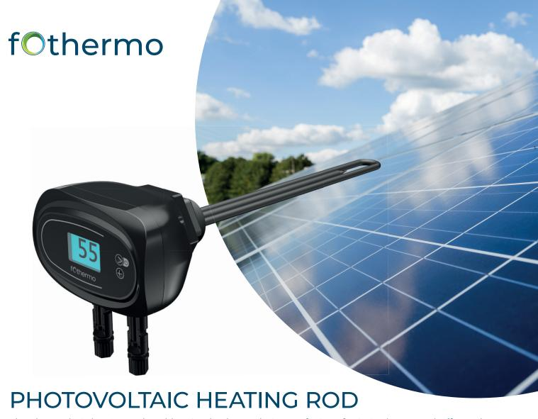
The photovoltaic heating rod enables simple photovoltaic retrofitting of existing hot water buffer tanks. The heating rod is screwed into a standard 1,5" thread. The photovoltaic support provides energy and cost savings for conventional hot water preparation via gas or oil heaters.
