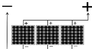
Connection of PV-modules in parallel configuration only!
