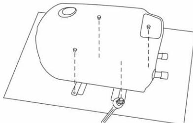
**IMPORTANT!** The Installation of the photovoltaic boiler is **only horizontally** possible.
