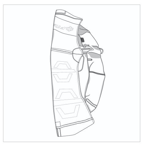
Fold up the first half of the wing, in between the bottom two handles.
